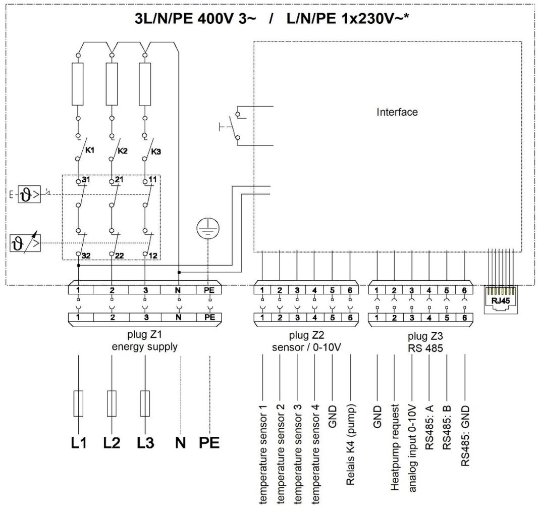
\* for single-phasing (1x230V~) L1, L2 and L3 use external jumper
