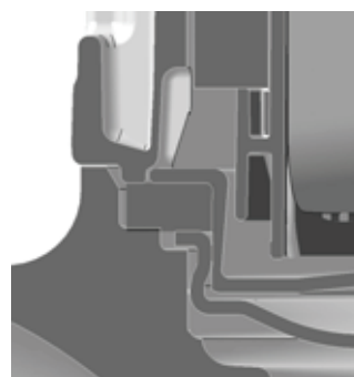
Fig. 37 Sectional drawing showing sealing principle of gasket
